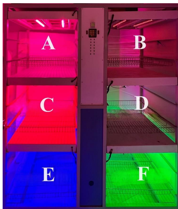
Fig. 1: Light shelf with six separate boxes. A: full spectrum light; B: far red; C: red light; D: UVA; E: blue light; F: green light
