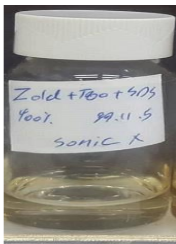
Figure 1. Evaluation of the stability of Zataria multiflora nanoemulsion prepared by spontaneous emulsification method with Tween 80 and SDS surfactants after 90 days.
