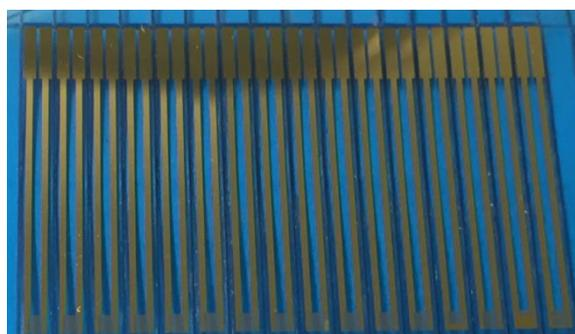
Fig. 1- Gold Interdigitated Thin Film Electrodes
