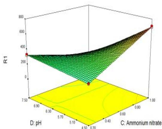
Fig. 2- Response surface plot describing effect of ammonium nitrate (g/l) and pH on GLA concentration ( $R_1$ )
